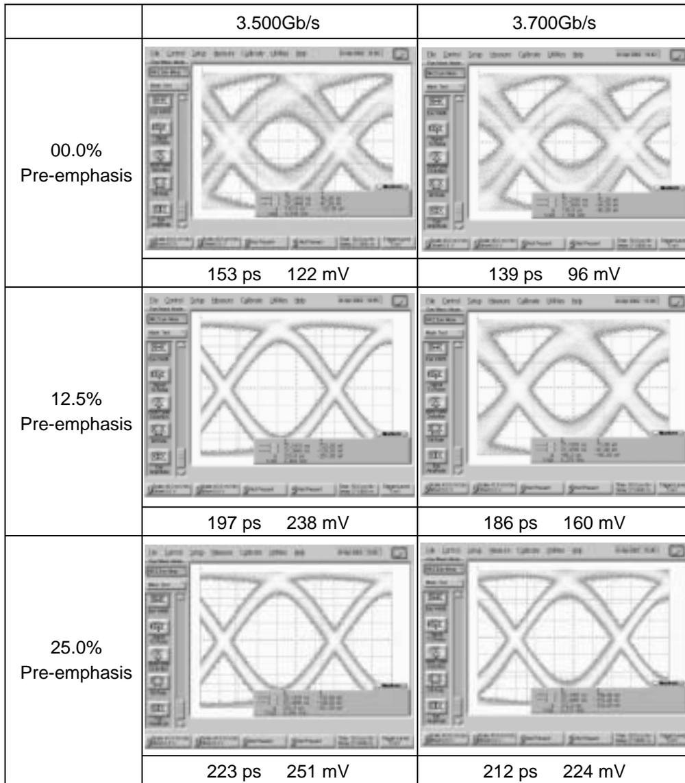
The eye-openings are smaller in the above Figure because of the higher data rates, where the path losses are greater. At these data rates 25% pre-emphasis must be used to achieve a comfortable margin above the 80 mV required eye-opening level.
