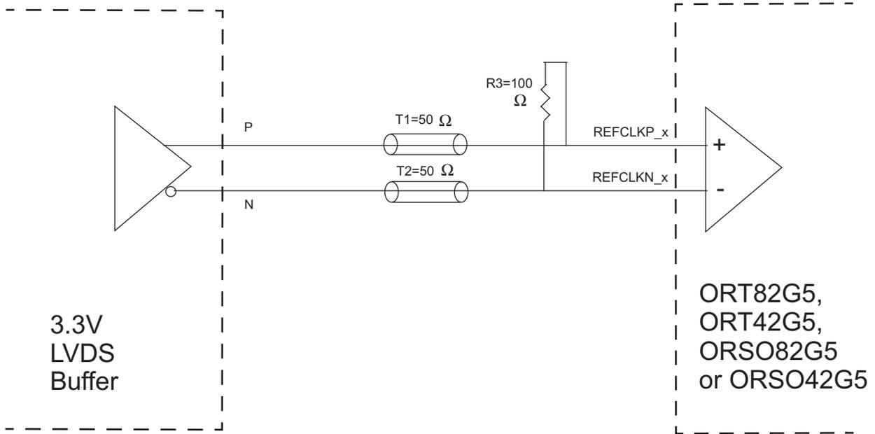
The standard LVDS output dc voltage is compatible with the ORT82G5, ORT42G5, ORSO82G5 and ORSO42G5 RefClk input, allowing a very simple interface circuit. The single termination resistor should minimize the possibility of system generated EM noise coupling into the reference clock signal.
