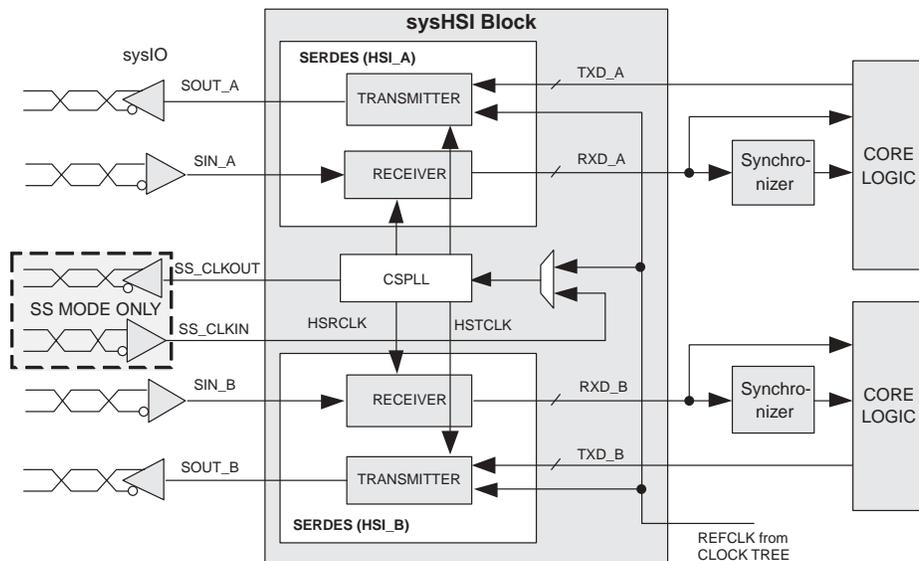
There is always a 10-bit wide data transmitted or received at the low speed side of the SERDES for both 10B/12B and 8B/10B modes. In 10B/12B encoding mode, the start bit(1) and stop bit(0) are added or removed within the sysHSI Block. In SERDES mode without encoding/decoding, (currently 8B/10B mode is supported), the encoding
