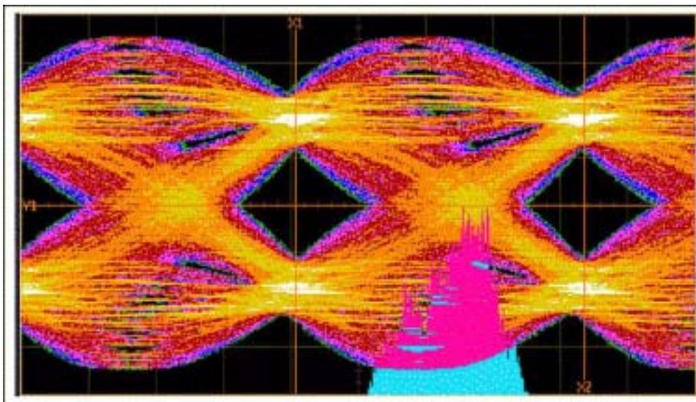
Note that Figure 4 also shows a density function of the waveform level transition crossings through the center (horizontal) axis, between the second and third eye openings.
