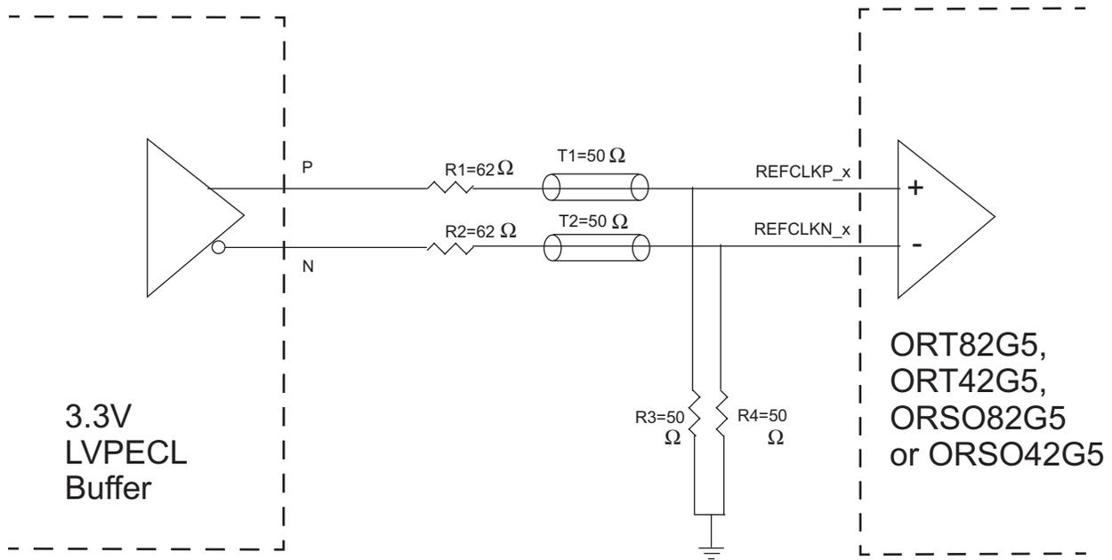
The dc coupling scheme from the 3.3V LVPECL clock signal buffer output allows a minimal number of discrete components in the interconnection circuit.
