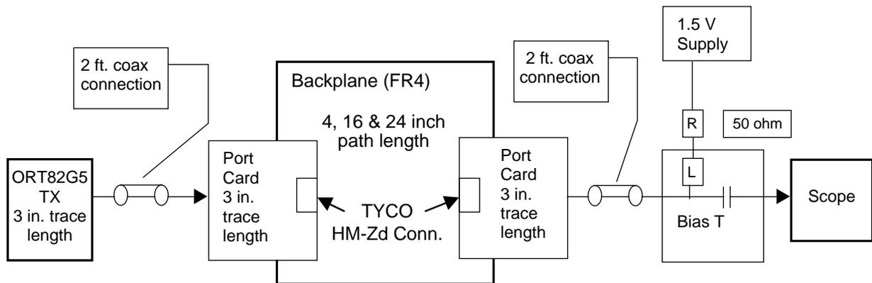
Figure 5 shows the test setup used for bit-error rate measurements discussed in this section.
