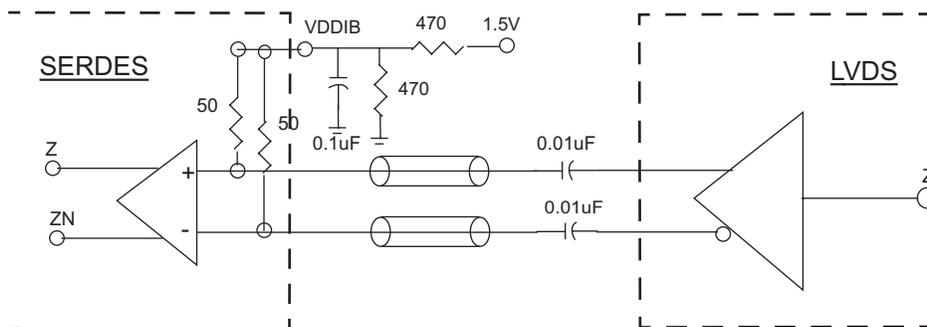
The signal coupling capacitors and resistive voltage divider circuit is added to translate the LVDS output signal to the center of the SERDES input voltage range. This will increase the receiver tolerance to common-mode input noise voltage, and provide a higher tolerance range to common-mode and system and ground noise. Note that nominal resistor and capacitor values are shown in Figure 3 and Figure 4. Optimum values will vary in each application.
