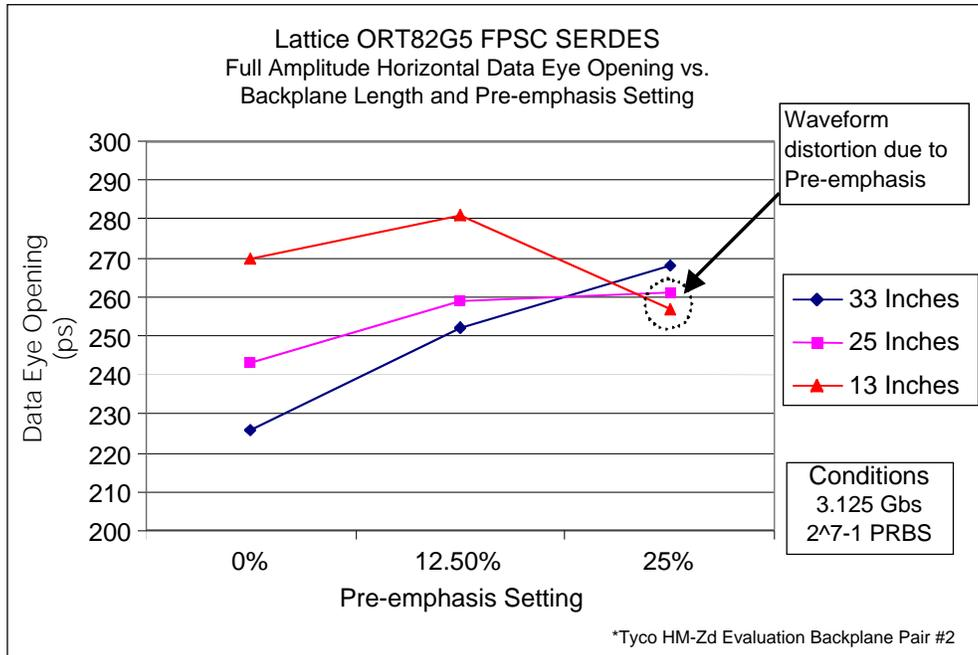
Figure 12. Pair 13 Eye-Opening vs. Pre-Emphasis and Trace Length
