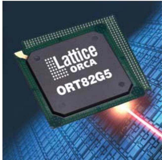
or across a backplane. The built-in clock recovery of the ORT82G5 and ORT42G5 allows higher system performance, easier-to-design clock domains in a multiboard system, and fewer signals on the backplane.
