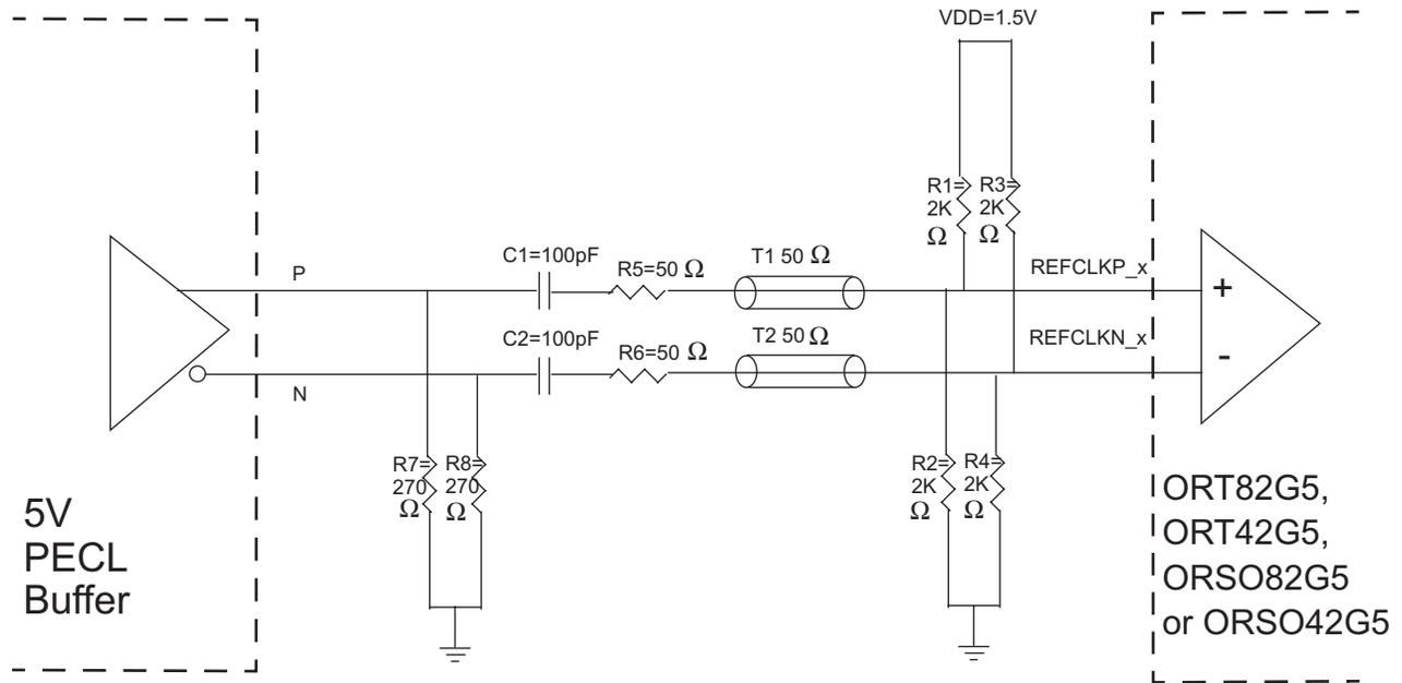
A conventional ECL source terminated configuration is used with ac coupling. Resistive voltage divider biasing of the Reference Clock input pins must be provided.
