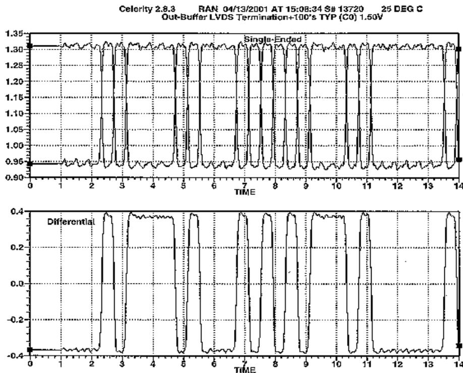
Figure 6 repeats the simulation of Figure 5, but under some worst case conditions. Extreme IC process parameters, low supply voltage, and 0 degree C temperature were assumed. The resulting waveforms in Figure 5 and Figure 6 are well within the acceptable operating range of a typical LVDS device. One of the important functions of circuit simulation is to verify correct operation while varying parameters and operating conditions over the expected range of variation.
