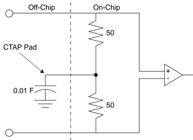
The center-tap is a virtual ground which may be ac-coupled to ground to increase receiver common mode noise immunity, as shown in the figure. Embedded LVDS output buffers also have on-chip 100 ohm\_ differential terminations, but do not have a center tap. These terminations have been shown to reduce near-end crosstalk significantly.
